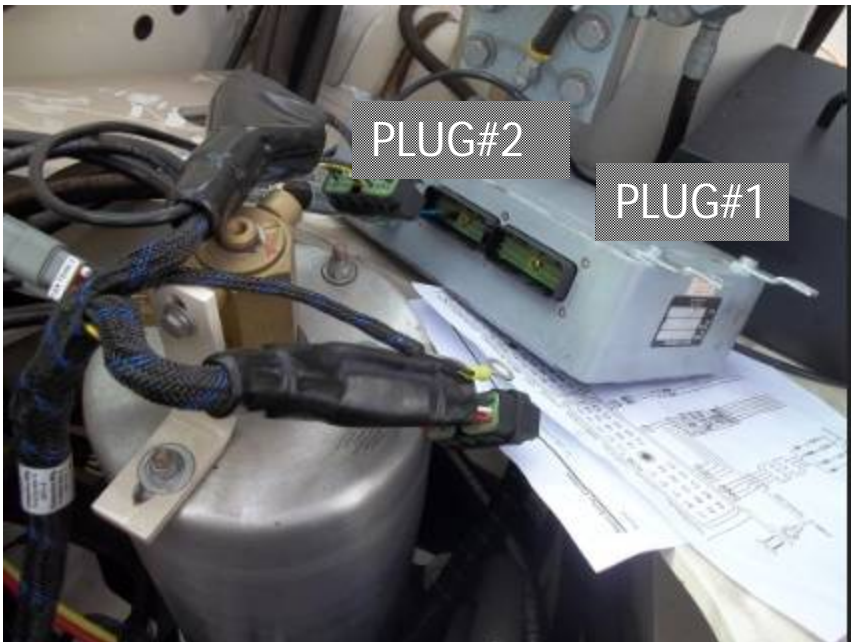
Pines: Delphi Metri-Pack 150 Series Terminal
